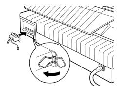
3. If your cable has a ground wire, connect it to the printer's ground connector as shown below.
