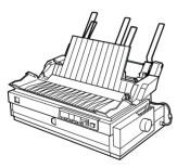
Connects to the high-capacity cut-sheet feeder to create a double-bin cut-sheet feeder. You can load up to 50 sheets of ordinary single-sheet paper in the second-bin cut-sheet feeder. For instructions on using this option, see page A-4.
