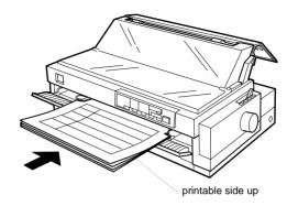
☐ You can load single-sheet multipart forms bound at the side only in the front slot. Insert this type of form in the front slot with the top edge first and the printable side up, as shown below.
