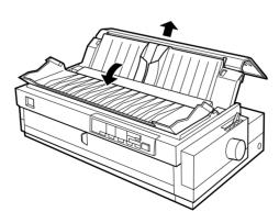
2. Set the paper release lever to the rear push tractor position. Also set the paper thickness lever (located under the printer cover) to the proper position for your paper's thickness.
