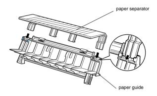
Make sure the paper guide cover is open as shown below. Attach the paper guide by sliding the slots on the bottom of the paper guide over the pegs behind the paper tension unit.
