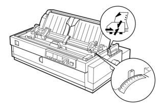
4. Release the left and right sprockets by pulling the sprocket lock levers forward.
