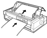
Load paper in the bottom slot printable side up (forward).
