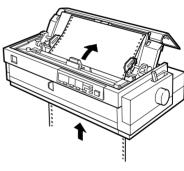
Before you load paper in the rear slot, remove the paper guide. Then load paper in the rear slot printable side down.
