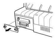
3. Slide the interface card along the slots on both sides of the interface compartment. Firmly push in the card to make sure the connector at the back of the interface card is fully inserted into the printer's internal socket. Then replace the screws and tighten them.
