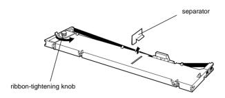
Hold the cartridge with the ribbon-tightening knob up. Fit the two front notches of the ribbon cartridge over the small pegs on each side of the printer as shown below. Then lay the cartridge flat.
