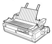
Feeds up to 150 sheets of paper, 25 plain bond envelopes, or 30 postcards into the printer without reloading. You can also load a stack of single-sheet multi part forms up to 15 mm  $(0.59 \, \text{in.})$  thick in this feeder. For instructions on using this option, see page A-4.
