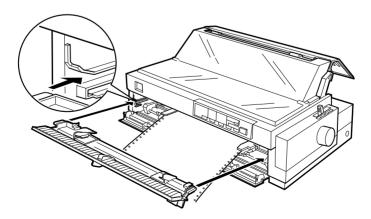
9. Slide the edge guides to the middle of the top paper guide. Make sure that the printer cover and the paper guide cover are closed.
