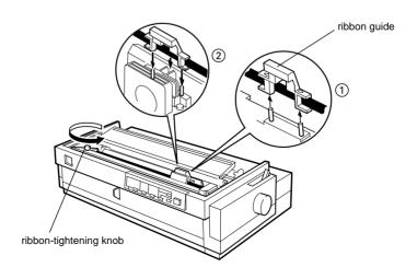
10. Turn the ribbon-tightening knob in the direction of the arrow to remove any slack in the ribbon, as shown above. Then slide the print head from side to side to make sure it moves smoothly.
