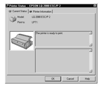
The Printer Status window contains two menus: Current Status and Printer Information. To open the menus, click the tabs at the top of the Printer Status window.
