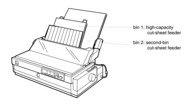
It is best to select the paper source in your application program because software settings usually override the printer's control panel settings. However, if you cannot select the paper source in your application, press the Tear Off/Bin button until the lights indicate the bin you want as shown below. When the printer receives data, it automatically loads paper from the bin you select.
