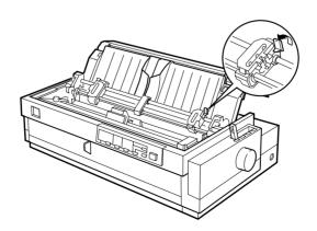
5. Slide the left sprocket to the left margin of the paper using the scale on the paper guide as a guide. (Printing starts at the arrow mark.) Then push the lever back to lock it in place.
