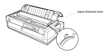
Use the following table to set the paper thickness lever to match the thickness of your paper.
