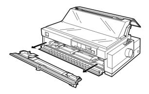
2. Set the paper release lever to the front push tractor position. Also set the paper thickness lever (located under the printer cover) to the proper position for your paper's thickness.
