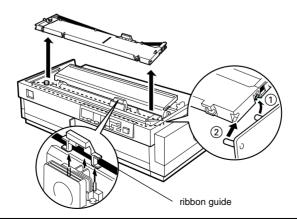
Remove the new ribbon cartridge from the package. Remove the separator from the middle of the ribbon cartridge and discard the separator. Then turn the ribbon-tightening knob in the direction of the arrow to remove any slack in the ribbon.
