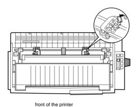
4. Slide the left sprocket to the left margin of the paper using the scale on the printer. (Printing starts at the "0" mark.) Then push the lever back to lock it in place.
