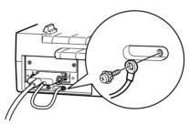
4. Plug the other end of the cable into the computer. (If the cable has a ground wire at the computer end, attach it to the ground connector at the back of the computer.)
