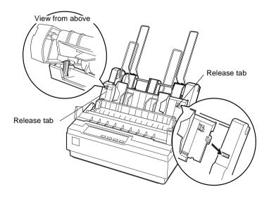
13. Slide the left edge guide to the center until it stops at the guide mark. Then slide the right edge guide to fit the size of paper you will use.
