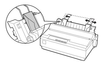
4. Slide a sheet of paper down firmly between the edge guides until it meets resistance. The printer loads the sheet automatically and begins printing the self test.
