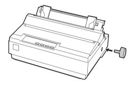
2. Push firmly on the paper-feed knob until it fits against the printer case.
