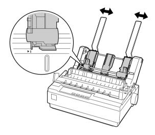
6. Pull the paper-set levers all the way forward until the edge guides retract and lock open to allow for paper loading.
