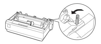
2. Release the sprocket units by pulling the sprocket locks forward.
