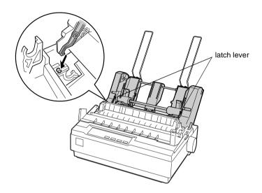
5. Slide the left edge guide so it is aligned with the triangle mark. Next, slide the right edge guide to roughly match the width of your paper. Slide the paper support midway between the edge guides.
