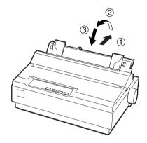
2. Hold one of the paper supports and push the tips into the notches on the edge guide.
