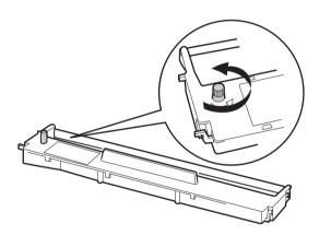
4. Insert the ribbon cartridge into the printer as shown; then press both sides of the cartridge firmly to fit the plastic hooks into the printer slots.
