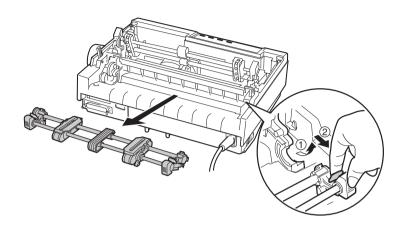
3. Move the tractor forward to the mounting slot at the top of the printer and tilt it into place as shown below. When you push the tractor onto the posts, you should feel the notches snap into place.
