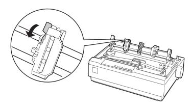
5. Insert the paper into the bottom paper slot or into the rear paper slot as shown below, and pull it up. Position the paper using the scale on the printer as a guide. The printer prints to the right of the position marked **0**.
