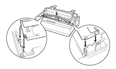
5. Use a pointed object, such as a ball point pen, to guide the ribbon between the print head and ribbon guide. Turn the ribbon-tightening knob to help feed the ribbon into place; it should not be twisted or creased.
