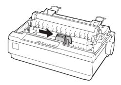
3. Turn the ribbon-tightening knob in the direction of the arrow to remove any slack from the ribbon so it is easier to install.
