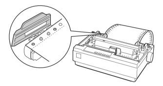
5. To separate the incoming paper from the printed paper, attach the paper guide by holding it horizontally and fitting its notches over the printer's mounting posts as shown below. Then slide the paper guide toward the front of the printer until you feel it click.
