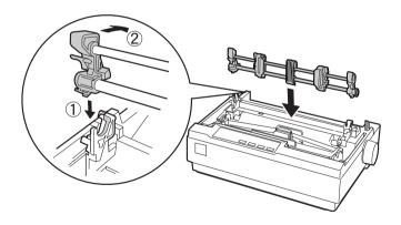
4. Release the sprocket units by pulling the sprocket locks forward.
