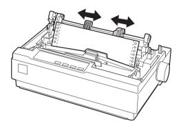
7. Make sure your paper has a clean, straight leading edge. Open the sprocket covers. Fit the first holes of the paper over the sprocket pins and then close the sprocket covers. Slide the right sprocket unit to remove any slack in the paper and then lock it in place.
