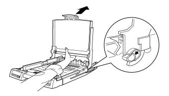
4. Lift the paper tray cover up and toward you so that the cover notches easily slide off the paper tray posts.
