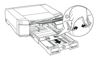
3. Align the right edge of the paper with the right edge guide and load the paper printable side down in the feed slot until it meets resistance.
