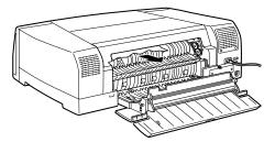
8. Open the rear manual feed slot cover and the printer cover. Gentry pull the jammed paper out.
