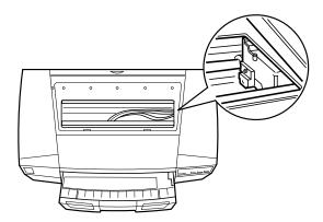
4. Remove all four of the ink cartridges and store them in separate plastic bags. Close the ink cartridge clamps and compartment covers.
