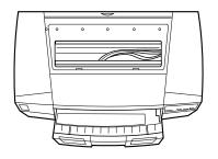
Warning: Be careful not to touch the gears inside the printer.
