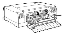
7. Gently pull the jammed paper out. If you are unable to remove the jammed paper, continue following these steps. If you can remove the jammed paper, go to step 9.
