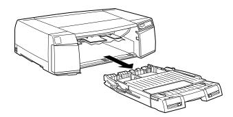
3. Gently pull the jammed paper out. If you are unable to remove the jammed paper, continue following these steps. If you can remove the jammed paper, go to step 9.
