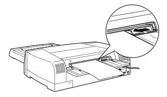
5. Align the right edge of the paper with the right edge guide, and load the paper printable side up in the rear feed slot until it meets resistance.
