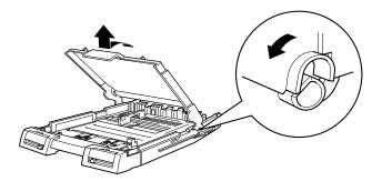
5. Lower the other paper tray cover so that the cover notches slide straight down and fit on the paper tray posts.
