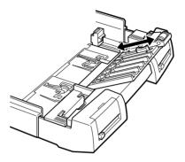
□ After paper is loaded, put the paper guide roller back in the paper tray.
