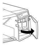
3. Lift up the ink cartridge clamp for the empty ink cartridge, then carefully pull the empty cartridge straight out of the printer.
