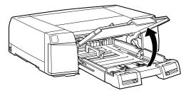
3. If you load Legal-size or larger paper, release the extension lock and pull out the paper tray extension completely.
