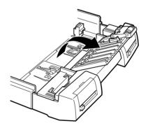
4008737 XXX-00  Set the roller position to match the paper size you are loading by sliding the switch. Set the roller to "Other" when loading paper other than A3 or Ledger size.
