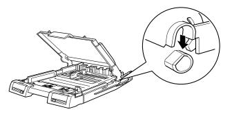
6. Move the paper tray cover to the upright position and make sure the cover notches click into place over the paper tray posts.
