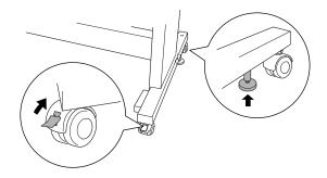
4. Carefully roll the printer to its new location. Relock the casters and extend the stabilizer knobs after moving.
