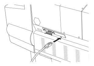
3. Connect the **E** end of the USB cable to your computer's USB port or a first tier USB hub port.
