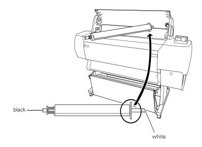
2. Insert the white end into the right mounting bracket inside the printer. You can use either the upper or lower bracket.
