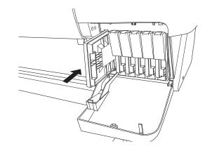
7. Push the cartridge clamp back up. Make sure the corresponding Ink Out light goes off. Then close the ink compartment cover.
