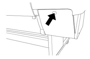
3. Locate the slot containing the empty ink cartridge (corresponding to the INK OUT light). Press down on the top of the clamp and pull it forward.
