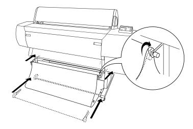
3. Release the front casters and retract the stabilizer knobs.
