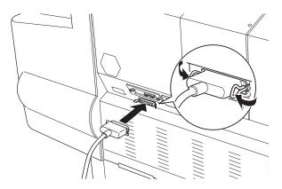
3. Plug the other end of the cable into the computer's parallel port.
