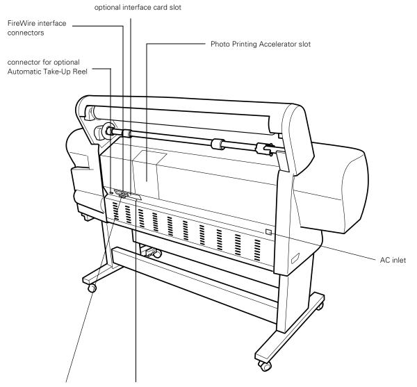
parallel interface connector USB interface connector
