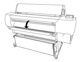
5. When REPLACE CUTTER appears on the display, you can open the casing. Push the side pin toward the back while pushing the front half of the paper cutter cover up.
