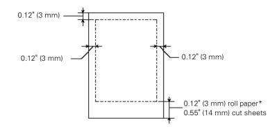
\* Default roll paper top and bottom margins are 0.59 inches (15 mm). You can set all margins to 0.12 inches (3 mm) or 0.59 inches (15 mm) using the control panel. See page 5-8 for instructions.
