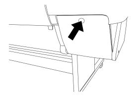
3. Push down on the top of the first cartridge clamp and pull it forward.
