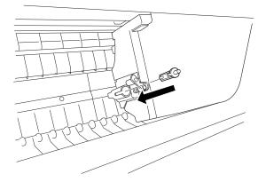
4. Push the side pin toward the back while pushing the front half of the paper cutter cover down to close the casing. Then release the side pin. CLOSE LOWER COVER appears on the display.
