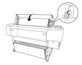
7. Press the **Pause** button. The print head moves and the paper feeds into printing position automatically. **READY** appears on the control panel display. (Even if you don't press **Pause**, the paper and printer will move into printing position automatically after 10 seconds.)
