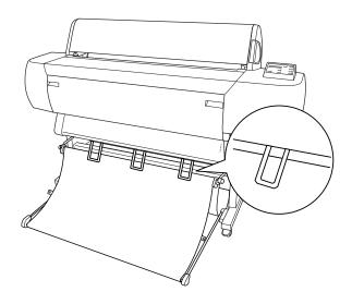
• If you have the paper hammock set up below the printer, extend the paper guides so that they rest on the back of the hammock.
