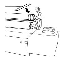
When you're not using the roll paper belt, keep it wound around the end of the spindle.
