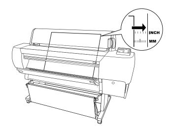
7. Align the board with the vertical row of holes at the paper exit.
