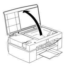
2. Place the original on the document table, with the side to be copied facing down. Make sure that the document is properly aligned.
