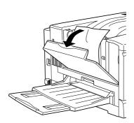
2. Remove all jammed paper. If paper has jammed at the top of the output path, gently lift it out. If it has jammed near the bottom of the output path cover, carefully pull it out of the printer.
