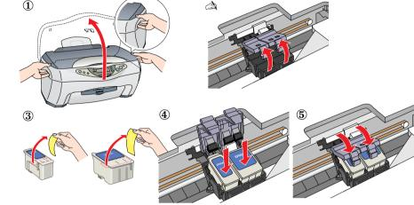
Install both ink cartridges. This product does not work unless both cartridges are installed properly.
