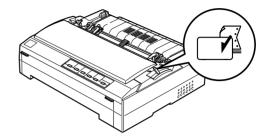
3. Release the left and right sprockets by pulling the blue sprocket lock levers forward.
