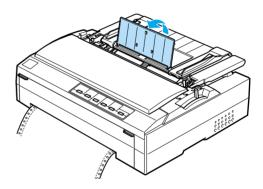
12. Turn on the printer. When the printer receives data, it automatically loads the paper and starts printing.
