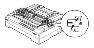
3. Release the sprockets by pulling the sprocket lock levers forward.
