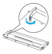
8. Hold the ribbon cartridge by its handle and insert it into the printer as shown below; then press both sides of the cartridge firmly to fit the plastic hooks into the printer slots.
