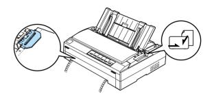
5. Load single sheets as described in "Loading Single Sheets" in the Reference Guide.
