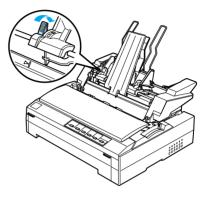
8. Push back the paper set levers to clamp the paper or envelopes against the guide rollers.
