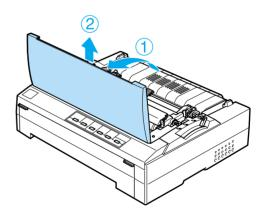
4. Press the tabs on each side of the paper tension unit upward, then lift the front of the unit and pull it up and out of the printer.
