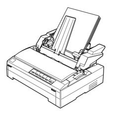
7. Adjust the right paper guide so that it matches your paper's width and lock it in place. Make sure the position of the guide allows the paper to move up and down freely.
