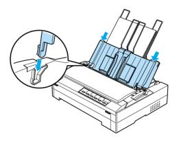
The cut-sheet feeder automatically loads paper when the printer receives data.
