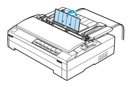
9. Turn on the printer. When the printer receives data, it automatically loads the paper and starts printing.
