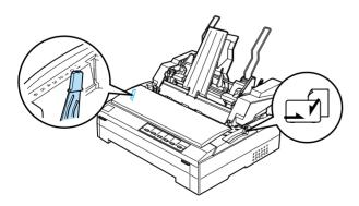
2. Pull the lock levers on the edge guides forward to release them.
