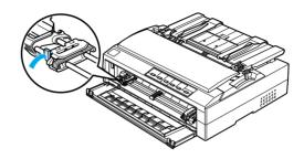
5. Slide the left sprocket approximately 12 mm (0.5 inch) from the far left position and pull the blue lever forward to lock it in place. Then slide the right sprocket to match the width of your paper, but do not lock it. Move the center support midway between the two sprocket units.
