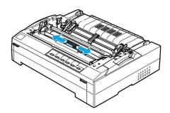
11. Reinstall the paper tension unit by lowering it onto the printer's mounting pegs. Then press down on both ends of the unit until it clicks into place.
