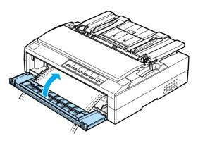
11. Make sure the paper guide is lying flat on the printer and the edge guides are open all the way to the left and right. Then raise the continuous paper support.
