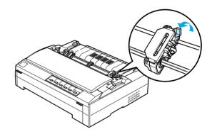
4. Slide the left sprocket approximately 12 mm (0.5 inch) from the far left position and push the blue lever back to lock it in place. Then slide the right sprocket to match the width of your paper, but do not lock it. Move the center support midway between the two sprocket units.
