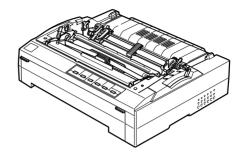
7. Remove the new ribbon cartridge from the package and turn the ribbon-tightening knob in the direction of the arrow to remove any slack from the ribbon so it is easier to install.
