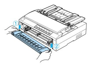
7. Make sure your paper has a clean, straight edge. Then open both sprocket covers and fit the first four holes of the paper, with printable side up, over the tractor pins.
