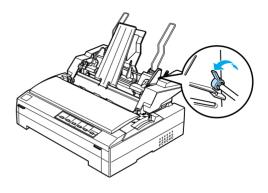
3. Slide the left paper guide until it is aligned with the triangle mark; then lock it in place by pushing back its lock lever. Next, slide the right paper guide to roughly match the width of your paper. Slide the paper support to midway between the paper guides.
