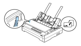
2. Slide the left paper guide of the cut-sheet feeder so it is aligned with the triangle mark. Next, slide the right paper guide to roughly match the width of your paper. Slide the paper support midway between the paper guides.
