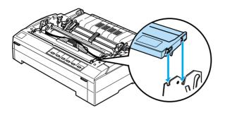
9. Use a pointed object, such as a ball point pen, to guide the ribbon between the print head and ribbon guide. Turn the ribbon-tightening knob to help feed the ribbon into place; it should not be twisted or creased.
