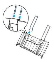
9. Install the paper guide with the attached stacker-support by fitting the notches on the paper guide straight down over the mounting posts on the printer. Slide the edge guides to the middle of your paper.
