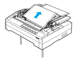
7. Fit four holes of the paper over the tractor pins on both sprockets. Then close the sprocket covers.
