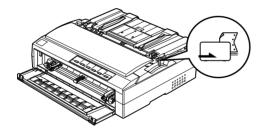
4. Release the left and right sprockets by pushing the blue sprocket lock levers backward.
