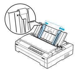
4. Insert a sheet of paper with the printable side down between the edge guides until it meets resistance. The printer feeds the paper automatically and is ready to print.
