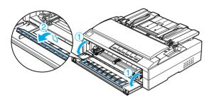
3. Set the paper release lever to the front push tractor position. Also set the paper-thickness lever (located under the printer cover) to the proper position for your paper's thickness. See "Paper-Thickness Setting" for instructions.
