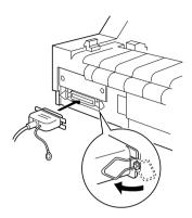
**4.** If your cable has a ground wire, connect it to the printer's ground connector as shown below.
