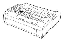
**6.** If a used ribbon cartridge is installed, grasp the cartridge by its handle and pull it straight up. Properly dispose of the used ribbon cartridge.
