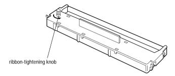
**8.** Hold the ribbon cartridge by its handle and push it firmly down into position; then press on both ends of the cartridge to make sure the plastic hooks fit into the slots.
