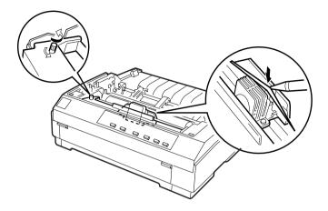
**10.** Slide the print head from side to side to make sure it moves smoothly. Also check that the ribbon is not twisted or creased.
