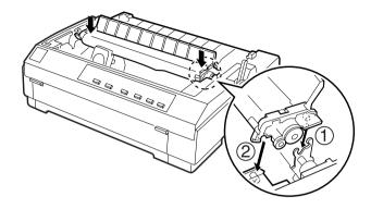
**12.** Replace the printer cover by first inserting the front tabs into the slots on the printer and then lowering the cover into place. Push it down until it clicks.
