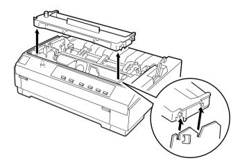
**7.** Remove the new ribbon cartridge from the package. Turn the ribbon-tightening knob in the direction of the arrow to remove any slack in the ribbon.
