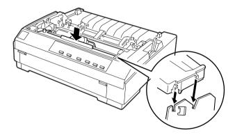
**9.** Use a pointed object, such as a ball point pen, to guide the ribbon between the print head and ribbon guide. Turn the ribbon-tightening knob to help feed the ribbon into place.
