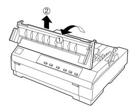
**4.** Push up the tabs on each side of the paper tension unit and lift the unit up and off the printer. Store the paper tension unit in a safe place.
