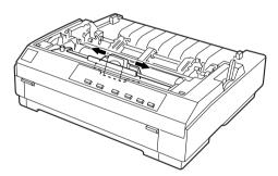
**11.** To replace the paper tension unit, lower it onto the printer's mounting pegs. Then press down both ends of the unit until it clicks into place.
