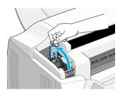
**9.** When installation is complete, press the **t** cleaning button and release quickly. The EPSON Stylus Scan moves the print head and begins charging the ink delivery system.
