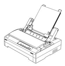
6. Adjust the right paper guide so that it matches your paper's width. Make sure the position of the guide allows the paper to move up and down freely.
