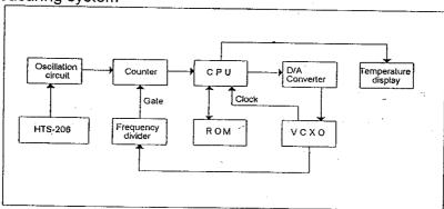
This measuring system has an internal clock, making it suitable for instances where an external high-precision oscillation source cannot be used.
