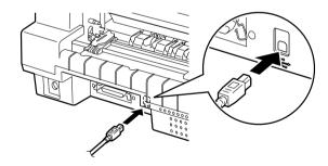
3. Connect the other end of the cable to the computer's USB port.
