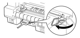
4. Plug the other end of the cable into the computer's parallel interface port.
