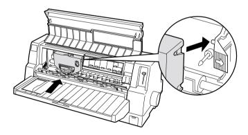
7. Turn the ribbon-tightening knob again to remove any slack in the ribbon so that the ribbon moves freely.
