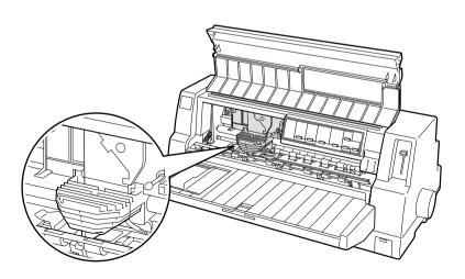
5. Remove the new ribbon cartridge from the package and turn the ribbon-tightening knob in the direction of the arrow to remove any slack from the ribbon so it is easier to install.
