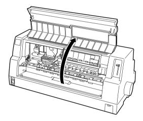
2. Slide the edge guide of the paper guide slightly to the center. Hold the paper guide horizontally with both hands, and slide the slots on both sides of it onto the mounting pegs in the printer as shown below. Then lower the paper guide until it locks into place.
