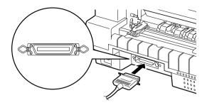
3. Squeeze the wire clips together until they lock in place on both sides of the connector.
