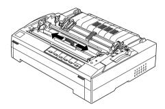
10. Reinstall the paper tension unit by placing it on the printer's mounting pegs and lowering it into place. Press down on both sides of the unit until it clicks into place.
