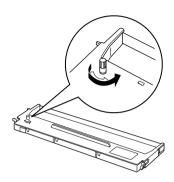
7. Hold the ribbon cartridge by its handle and insert it into the printer as shown below; then press both sides of the cartridge firmly to fit the plastic hooks into the printer slots.
