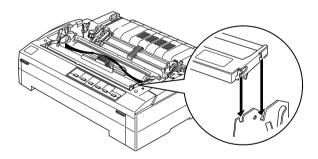
8. Use a pointed object, such as a ball point pen, to guide the ribbon between the print head and ribbon guide. Turn the ribbon-tightening knob to help feed the ribbon into place; it should not be twisted or creased.
