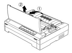
4. Press the tabs on each side of the paper tension unit upward, then lift the front of the unit and pull it up and out of the printer.
