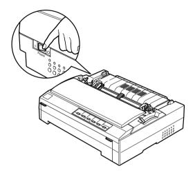
2. Check the label on the back of the printer to make sure the voltage required by the printer matches that of your electrical outlet. Also make sure the shape of the plug on your printer's power cord matches the shape of your electrical outlet.
