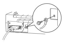
4. Plug the other end of the cable into the computer's parallel interface port. (If there is a ground wire at the end of the cable, attach it to the ground connector at the back of the computer.)
