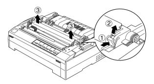
5. Make sure the print head is not hot; if it is, let it cool for a few minutes before touching it. Then slide the print head to the middle of the printer by hand.
