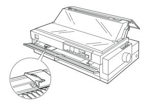
4. Set the paper release lever to the single-sheet position. Also set the paper thickness lever (located under the printer cover) to the proper position for your paper's thickness. (See the table on page 3-3.)
