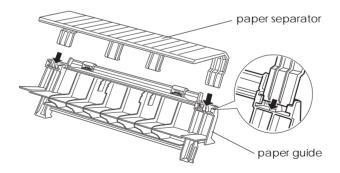
2. Make sure the paper guide cover is open as shown below. Attach the paper guide by sliding the slots on the bottom of the paper guide over the pegs behind the paper tension unit.
