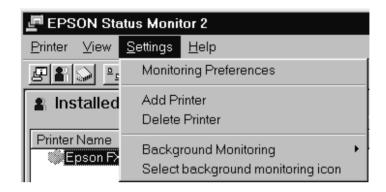
☐ Monitoring Preferences Opens the Monitoring Preferences dialog box, where you can adjust the monitoring interval and make background monitoring settings for the selected printer. For more information, see "Turning on background monitoring" on page 6-11.
