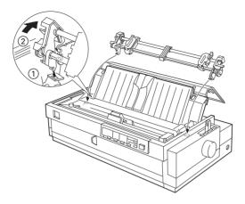
You are now ready to load continuous paper onto the pull tractor as described in the next section. To remove the pull tractor, see page 2-33.
