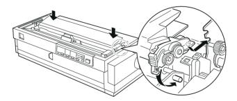
6. Replace the paper guide and printer cover. Then close the paper guide cover.
