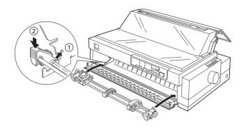
You are now ready to load continuous paper onto the front push tractor as described in the next section. To remove the tractor, see page 2-16.
