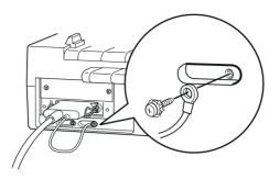
4. Plug the other end of the cable into the computer. (If the cable has a ground wire at the computer end, attach it to the ground connector at the back of the computer.)
