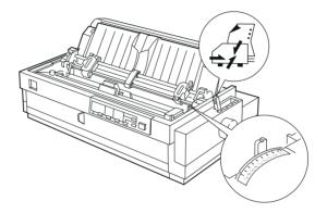
4. Release the left and right sprockets by pulling the sprocket lock levers forward.
