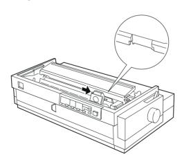
If a used cartridge is installed, grasp the cartridge and pull it slightly forward and up; the ribbon guide snaps away from the metal pins behind the print head. Properly dispose of the used ribbon cartridge.
