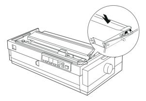
9. Lift the ribbon guide of the ribbon cartridge (①) and insert it firmly over the metal pins behind the print head (②). Make sure the ribbon is not twisted or creased and that it is in place behind the print head. Press down the guide until it clicks into place.
