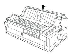
2. Set the paper release lever to the rear push tractor position. Also set the paper thickness lever (located under the printer cover) to the proper position for your paper's thickness.
