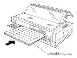
☐ You can load multi-part forms bound at the side only in the front slot. Insert this type of form in the front slot with the top edge first and the printable side up, as shown below.
