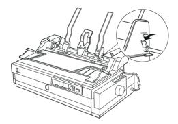
4. Holding the lower portion of the left paper guide, slide it until it is aligned with the arrow mark on the back of the center support. Then push the left lock lever backward to lock it in place. Holding the lower portion of the right paper guide, slide it to match the width of your paper, but do not lock it.
