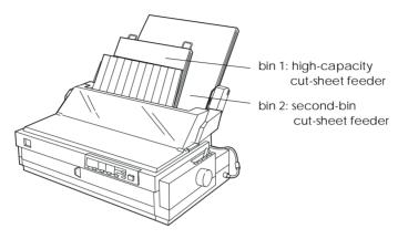
It is best to select the paper source in your application program because software settings usually override the printer's control panel settings. However, if you cannot select the paper source in your application, press the Tear Off/Bin button until the lights indicate the bin you want as shown below. When the printer receives data, it automatically loads paper from the bin you select.
