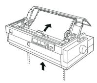
Before you load paper in the rear slot, remove the paper guide. Then load paper in the rear slot printable side down.
