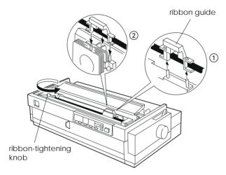
10. Turn the ribbon-tightening knob in the direction of the arrow to remove any slack in the ribbon as shown above. Then slide the print head from side to side to make sure it moves smoothly.
