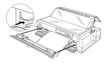
9. Slide the edge guides to the middle of the top paper guide. Make sure that the printer cover and the paper guide cover are closed.
