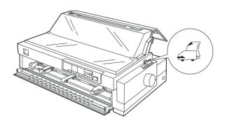
3. Release the left and right sprockets by pushing the sprocket lock levers backward.
