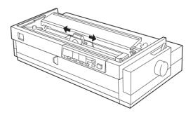
11. Replace the printer cover by first inserting the front tabs into the slots on the printer and then lowering the cover until it clicks into place.
