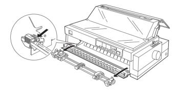
5. Replace the front paper guide by sliding it along the printer's mounting slots until it locks in place. Then close the front paper guide.
