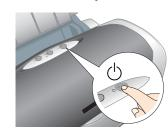
Make sure that the CD/DVD guide is closed when turning on the printer.
