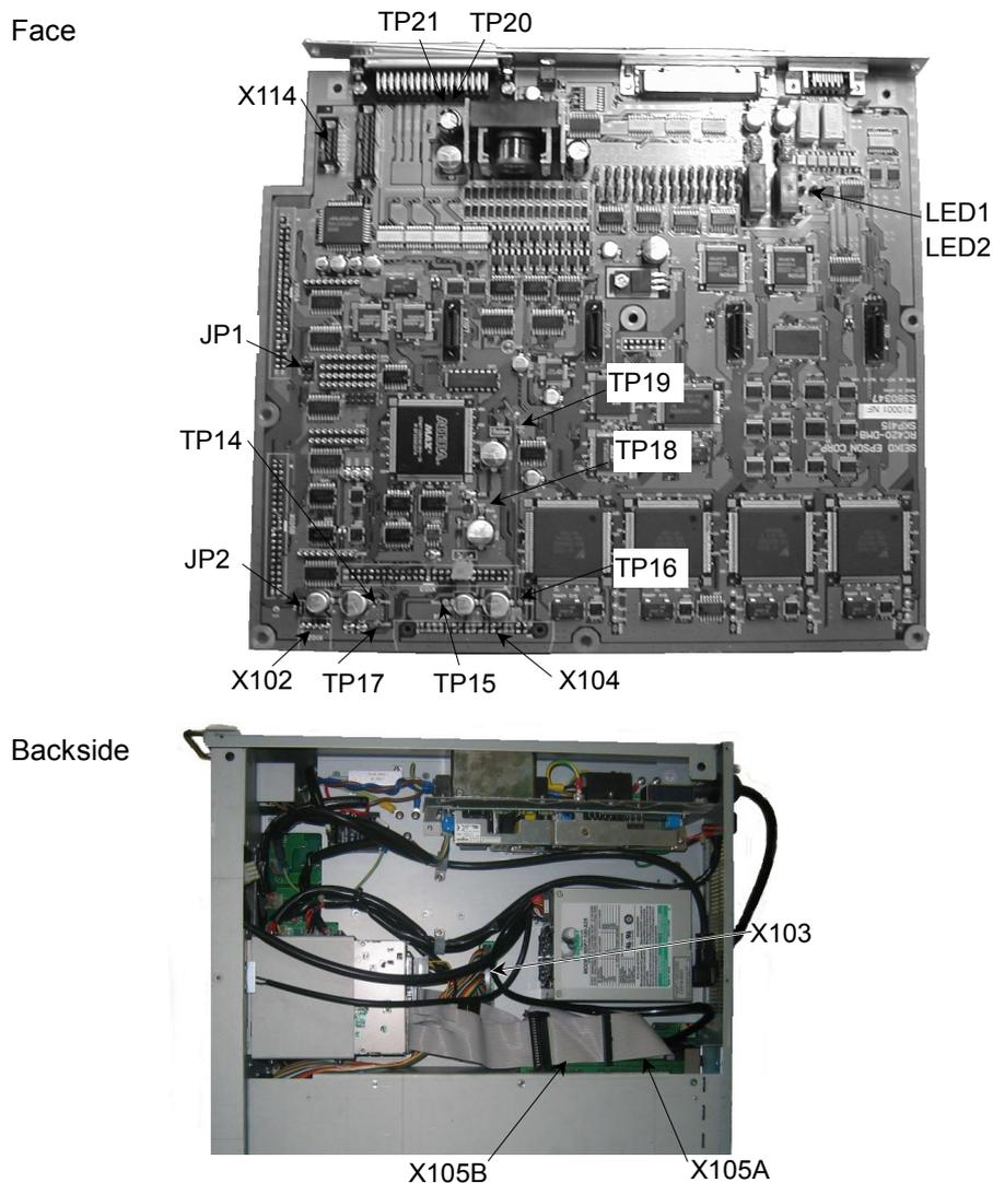
The test pins for voltage check
