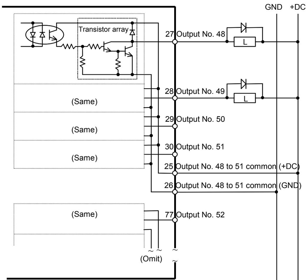
Rated Output Voltage : + 12 V to 24 V  $\pm 10\%$
