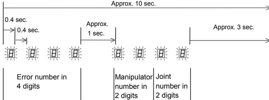
The above mentioned cycle (which lasts approximately 10 seconds) repeats and is displayed until the error is canceled or the power is OFF.
