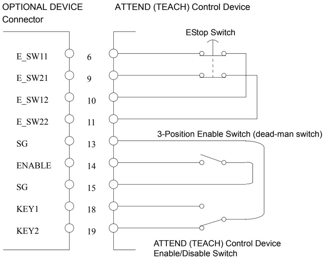
**NOTE** The 3-position enable switch is available when the ATTEND (TEACH) control device is enabled. The Emergency Stop switch is always available whether the ATTEND (TEACH) control device is enabled or disabled.
