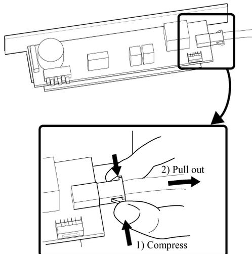
(14) Disconnect the flat cables (X104, X114) that connect to DMB.
