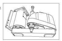
(2) Secure the base to the wall with six bolts.
