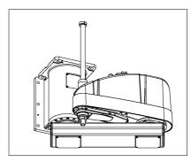
(2) Secure the base to the wall with six bolts.
