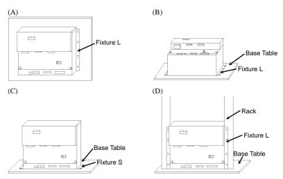
There are two types of fixtures. Mount the fixture to the Controller with the four attached screws.
