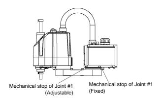
\* The different mechanical stop positions from Table Top mounting are indicated for Multiple mounting.
