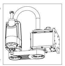
(2) Secure the base to the wall with four bolts.
