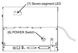
\* POWER switch is not available for RC180-UL. Instead, turn ON the external disconnecting means.
