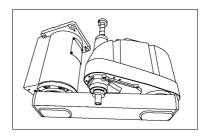
(2) Secure the base to the ceiling with four bolts.
