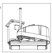
(2) Secure the base to the ceiling with four bolts.
