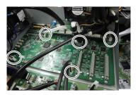
(7) Remove the DMB mounting screws ( $\times 15$ ).
