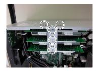
(5) Mount the output cable of each axis of the MDBs.
