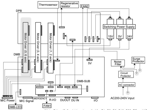
(Motor Driver (5, 6 axis) is not supplied for G1, G3, G6, G10, G20, RS and X5.)
