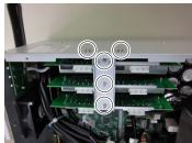
(6) Remove the MDB clamp 2.(Mounting screw × 2)
