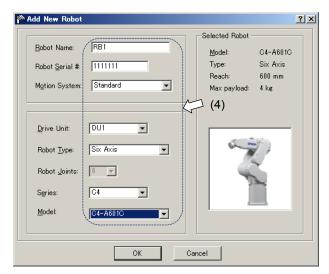
(4) Enter the following items by referring to the *RC700DU Robot System Hofs Data Sheet* (hereinafter referred to as Hofs sheet) which is included with shipment.
