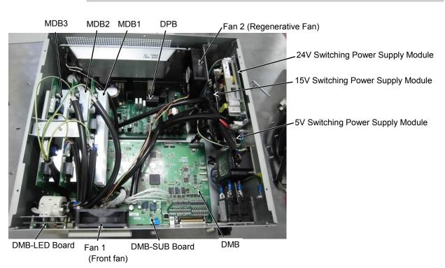
(MDB3 is not supplied for G1, G3, G6, G10, G20, RS and X5.)
