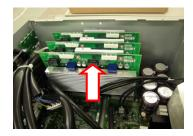
MDB Installation (1) Install the MDB clamp 3. (Mounting screw × 2)
