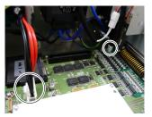
(10) Remove the DMB mounting screws ( $\times$ 14).
