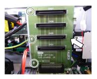
(7) Remove five screws on the side of the chassis.
