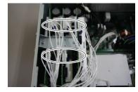
(5) Remove the MDB clamp 1. (Mounting screw ×5)
