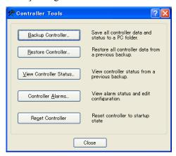
(2) Click the <Controller Alarms> button and display the [Controller Alarms] dialog box.
