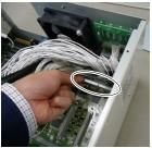
MDB Installation (1) Install the MDB clamp 3. (Mounting screw ×2)
