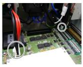
RC700-A: Connect the twelve connectors to the DMB.
