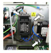
(8) Mount the five screws on the side of the chassis.
