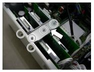
(6) Remove the MDB clamp 2. (Mounting screw ×2)
