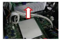
(8) Remove the MDB clamp 3. (Mounting screw ×2)
