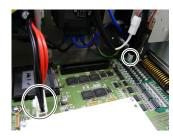
RC700-A: Remove the twelve connectors from the DMB.
