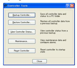
(2) To check the controller maintenance information, click the <Maintenance> button and display the [Maintenance] dialog box.
