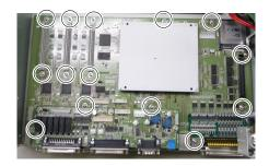
(6) RC700: Connect the five connectors to the DMB.
