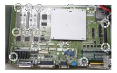
(6) RC700: Connect the five connectors to the DMB.
