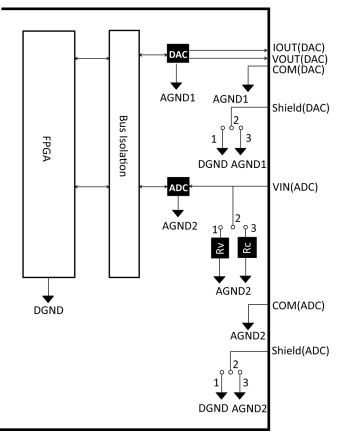
Rv: Voltage Input Terminating Resistance (100k $\Omega$ ), Rc: Current Input Terminating Resistance
