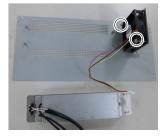
Regenerative Fan(1) Fix the new fan to the fan fixing plate. (Mounting screw  $\times$ 2) Installation
