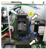
(9) RC700: Remove the five connectors from the DMB.
