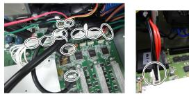
(10) Remove the DMB mounting screws ( $\times$ 14).
