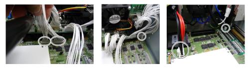
RC700-A: Remove the twelve connectors from the DMB.
