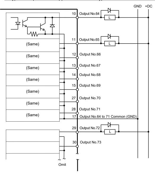
Typical Output Circuit Application 1: Sink Type
