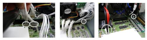
RC700-A: Connect the twelve connectors to the DMB.
