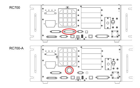
NOTEWhen nothing is connected to the TP port, Emergency Stop status occurs in the Controller.Image: Second status occurs occurs in the Controller.Image: Second status occurs o
