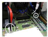
(7) Mount the fixing plate of the DMB-OPTION board.
