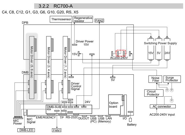
(Motor Driver (5, 6 axis) is not supplied for G1, G3, G6, G10, G20, RS and X5.) (Connecters in the red dotted line work properly in any order.)
