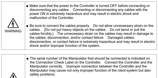
When connecting the Manipulator to the Controller, make sure that the serial numbers on each equipment match. Improper connection between the Manipulator and Controller may not only cause improper function of the robot system but also serious safety problems. The connection method varies with the Controller used. For details on the connection, refer to the Controller manual.
