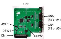
Switch and Jumper Configuration Set DSW1, DSW2 and JMP1. CN3 is all open.
