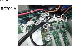
(5) Remove the screws fixing the DMB-SUB board to the front side plate.
