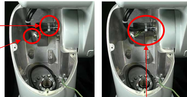
Arm #1 Front Cable Fixing Plate
