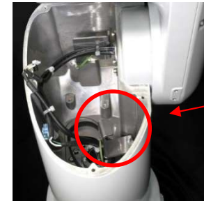
Arm #1 Cable Fixing Plate
