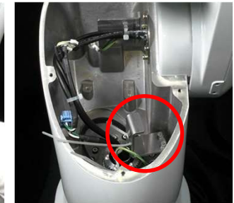
Arm #1 Cable Fixing Plate & Cable Tie
