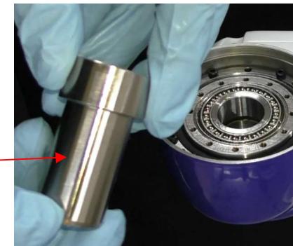
Joint #6 Centering Jig
