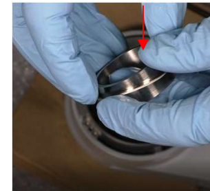
Wave washer Centering Jig
