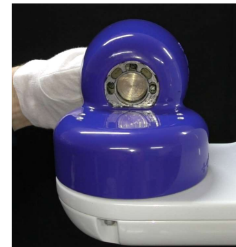
Joint #6 Centering Jig
