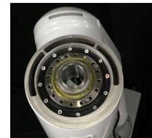
Wave washer confirmation point
