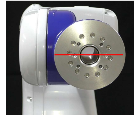
Correct 0 pulse position
