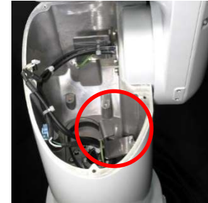
Arm #1 Cable Fixing Plate
