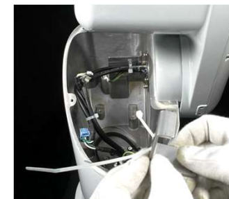
Arm #1 Cable Fixing Plate & Cable Tie
