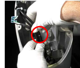
Arm #1 Cable Fixing Plate & Cable Tie
