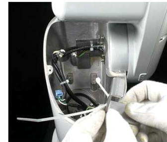
Arm #1 Cable Fixing Plate & Cable Tie
