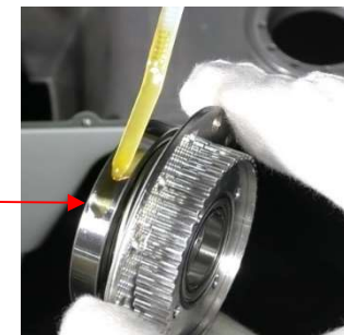
Joint #5 Reduction Gear Pulley & Bearing Unit
