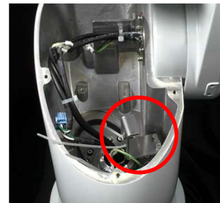
Arm #1 Cable Fixing Plate & Cable Tie
